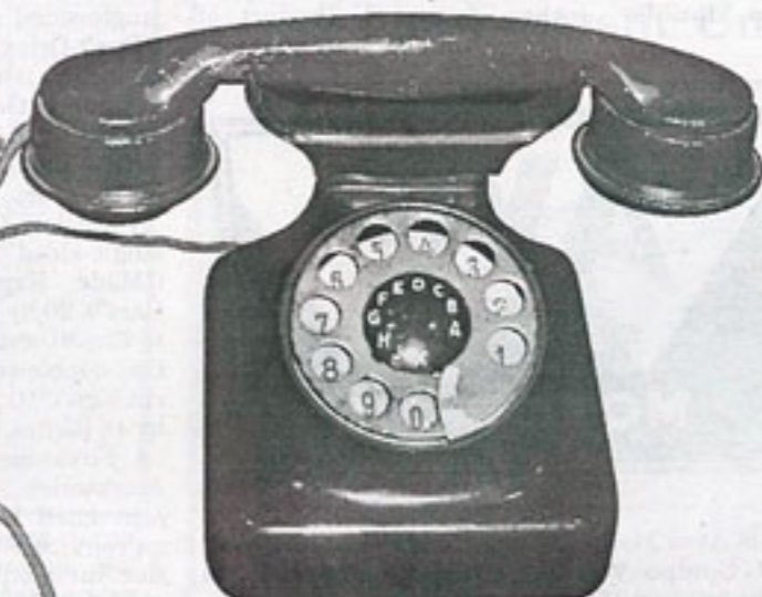
This Bakelite telephone handset, circa 1910-1920, Sweden, of Bakelite, metal and cotton, was made by Ericsson & Co. A.B., Stockholm.
