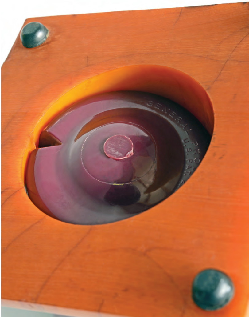
Figure 3. Bottom view shows protuberance on the base and notch and sprue on the thermoplastic tumbler bottom
